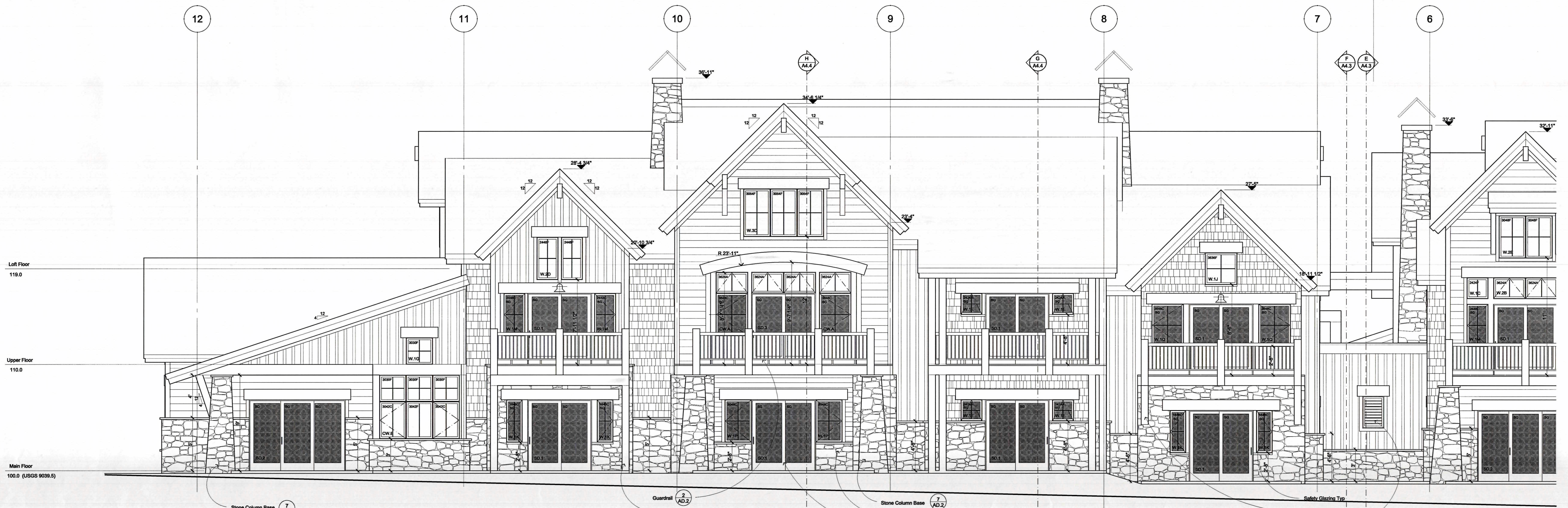
Stone Column Base Guardrail Vinyl Sliding Patio Doors Stone Column Base Stone Veneer and Cap Safety Glazing Typ End Knee Brace Mechanical Louver Verify Size and Location with Mechanical Design Main Floor USGS 9038.5 Main Floor USGS 9038.5 SOUTH ELEVATION SCALE: 1/4" = 1'-0"
